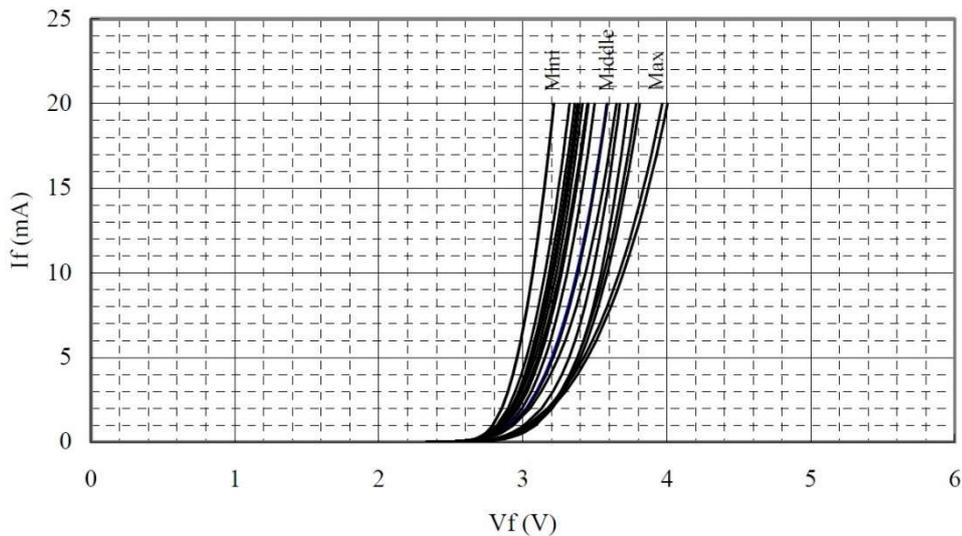
Figure 2. Forward Voltage - Forward Current
