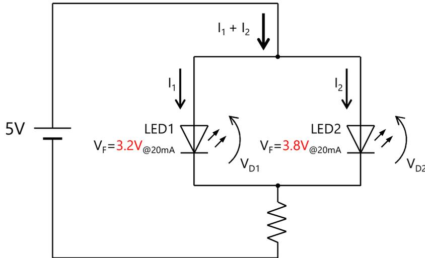
Figure 3. Circuit Diagram
